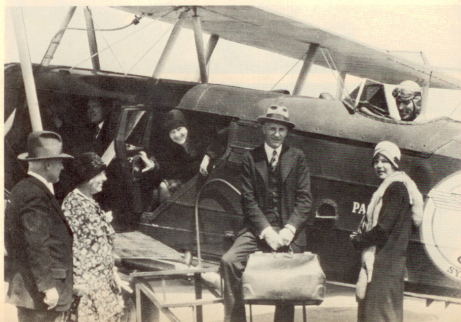
Passengers board a Boeing 40B-4 for 22½-hour San Francisco-Chicago flight. Note the loading ramp and separate doors for the two sections of the four-place cabin.
