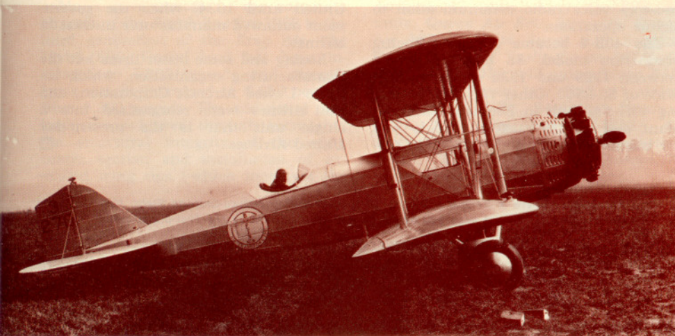
Improved 1927 Model 40A, with steel-tube fuselage and air-cooled Pratt and Whitney Wasp engine. Mail hold is between pilot's cockpit and two-place passenger cabin between the wings. Photos from The Boeing Company
